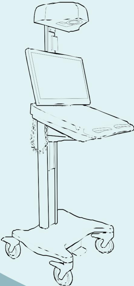
**Height:** From 40 inches /101.6 cm to 64.5 inches / 163.8 cm, height adjustment by means of a foot pedal with gas spring assisted control
